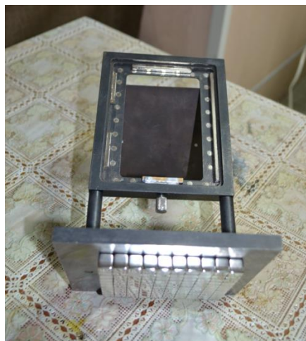
Figure 7. A holder with a podium made of neodymium magnets.
