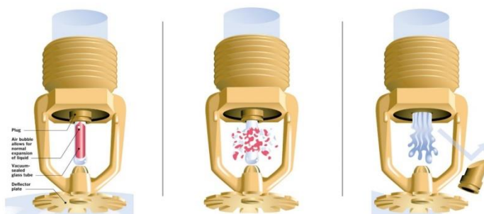
Picture 1. The moment of operation of the sprinkler with the socket "down".
