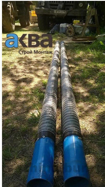
Figure 1. Two-string well with a coarse filter.
