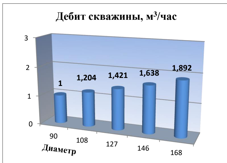
Figure 2. Histogram of the well flow rate depending on the diameter of the filter part in m 3 /h
