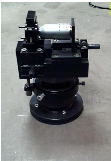
Figure 2. A spatial filter with a micrometric screw at the bottom.
